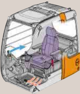
* Illustration shows a sample of the air flow during bi-level control.
